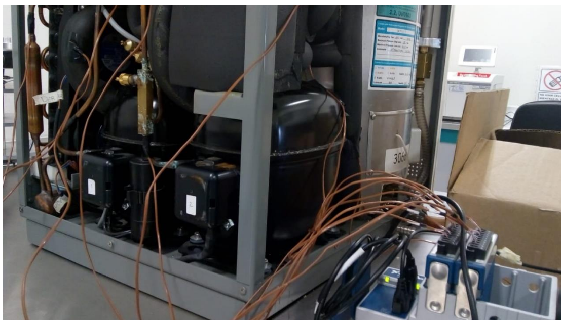
Figure 18. Experimental setup of the lyophilization device.
