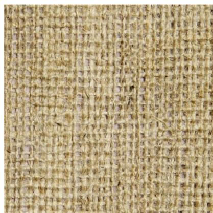
Figure 2. Bidirectional jute fabric
