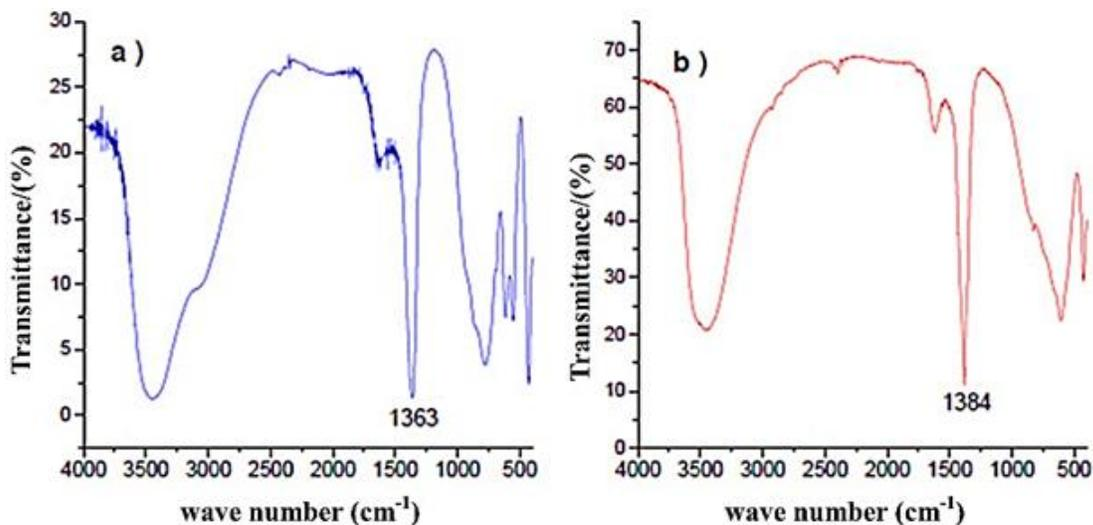
Figure 2. Infrared spectra of fresh LDH ZnAl-X. a) ZnAl-CO<sub>3</sub> and b) ZnAl-NO<sub>3</sub>.
