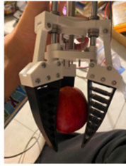
Figure 8. Experimental grasping tests using the fabricated gripper.
