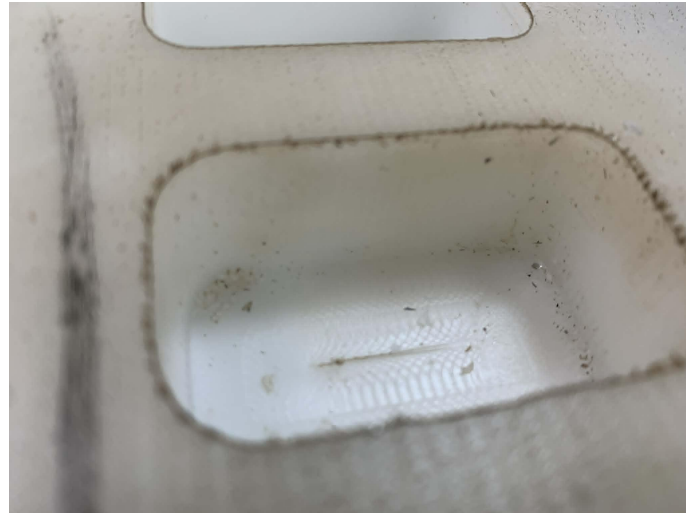
Figure 6. Balanced Pareto-optimal solution (shortest time, lowest force, poor surface).
