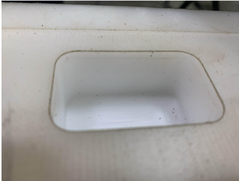
Figure 5. CAM-recommended baseline (smooth surface, long time, over-cut).
