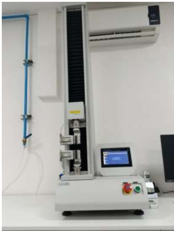
Figure 1. Universal testing machine GBD-2 Electronic Tensile Tester . (Source: Own elaboration).
