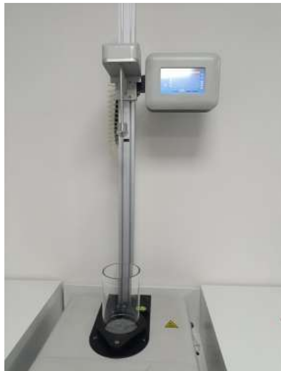
Figure 2. Impact machine GBD-12 Falling Dart Impact Tester . (Source: Own elaboration).
